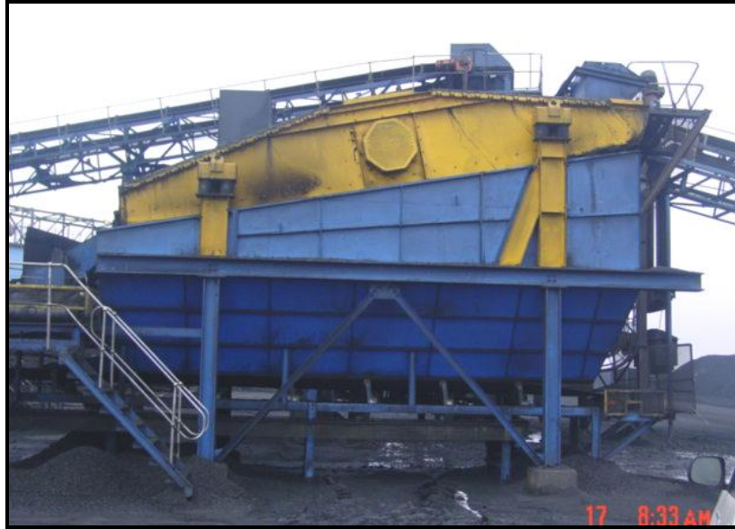
Figure 6: The Bivitec Screen at New Clydesdale Colliery
