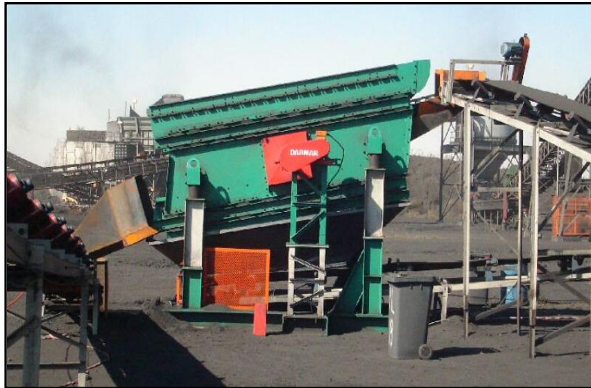
Figure 10: Bivitec screen test unit at Leeuwpan Coal Mine
